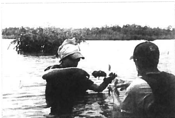
Figure 4. Photograph of acquiring the marine sediment samples at Chan b'i using a stainless steel knife and placing the sediment into Whirl-pak bags (photo by H. McKillop).
